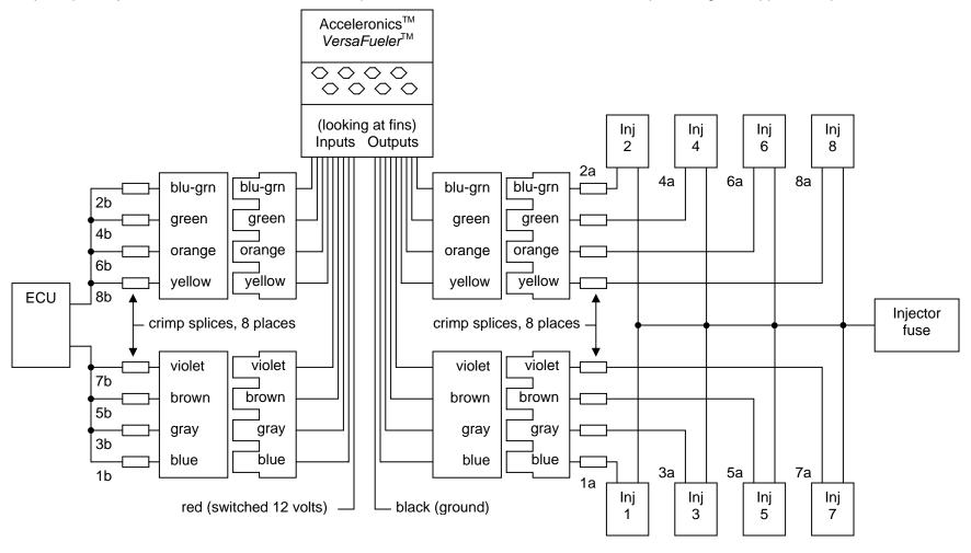
Step 4, attach the black wire ring terminal to a clean, shiny ground such as an engine or chassis bolt.
